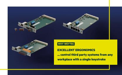
The WEYTEC IP Input / Output (IP I/O) cards receive, distribute and forward events within a WEYTEC KVM matrix system. IP I/O cards provide interfaces between WEYTEC IP devices and third party peripherals. In combination with a smartTOUCH keyboard or a WDP system, IP I/O cards detect incoming events and trigger outgoing events, interacting with visualization solutions, communication and radio systems, building management technology and more.
