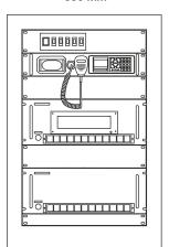
The Barrett 2075 500W P/N BC207505 is installed into a 20U rack unit weighing 92 kg with a depth of 700 mm. It ships as a complete unit including 19' rack mounting kits and blanking plates and all necessary cables and hardware ready for operation.
