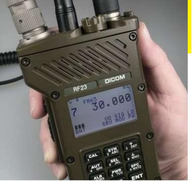
RF23 handheld multiband transceiver with increased resistance against radio-electronic warfare intended for squad/team, platoon and company operation is part of the RF20 tactical radios family.
